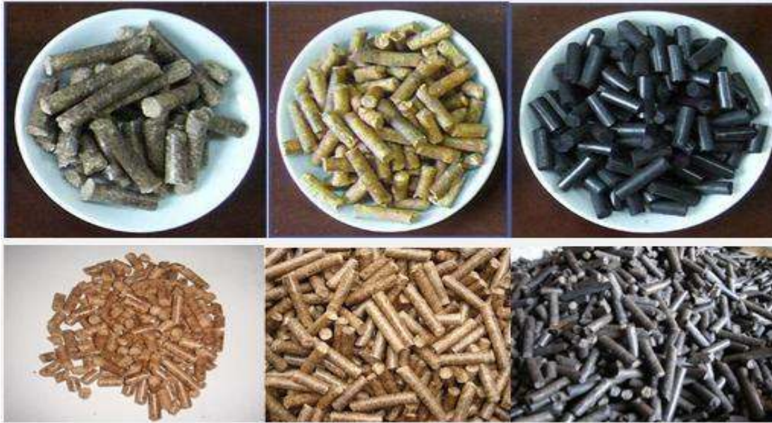
Fig. 27 Different color bamboo pellets productioned under different production temperature
